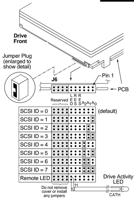
**Figure 3a. Model "N" drive ID Select and LED connection**
