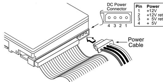
**Figure 5. Power connection to drive**
