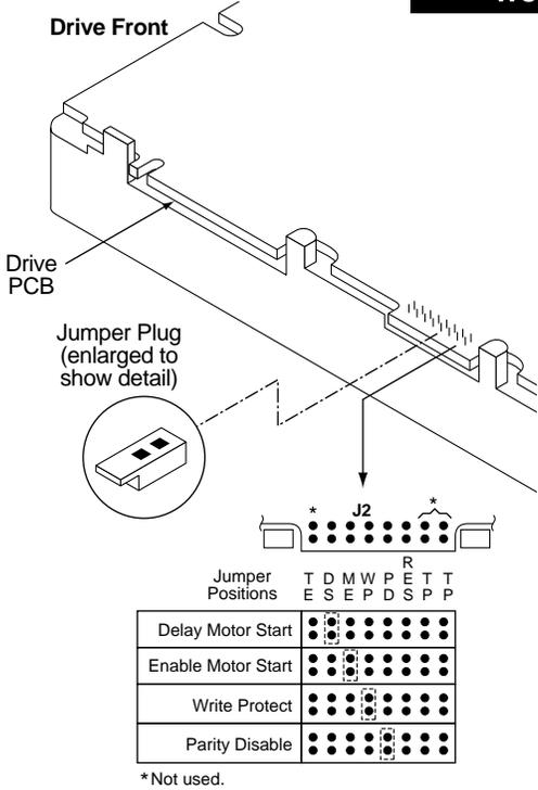
**Figure 3e. Model "WC" drive configurator, option select**
