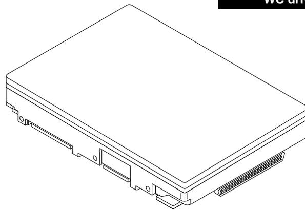
**Note:** This drive model plugs directly into a backplane connector and therefore uses no cables.
