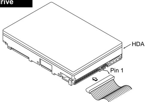
**Figure 4b. Sixty-eight pin connection to drive**
