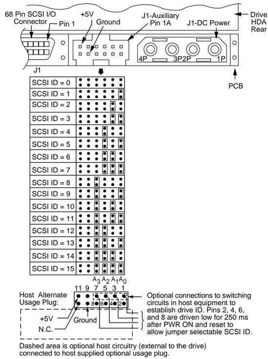
**Figure 3c. Model "W" drive ID select and LED connection**
